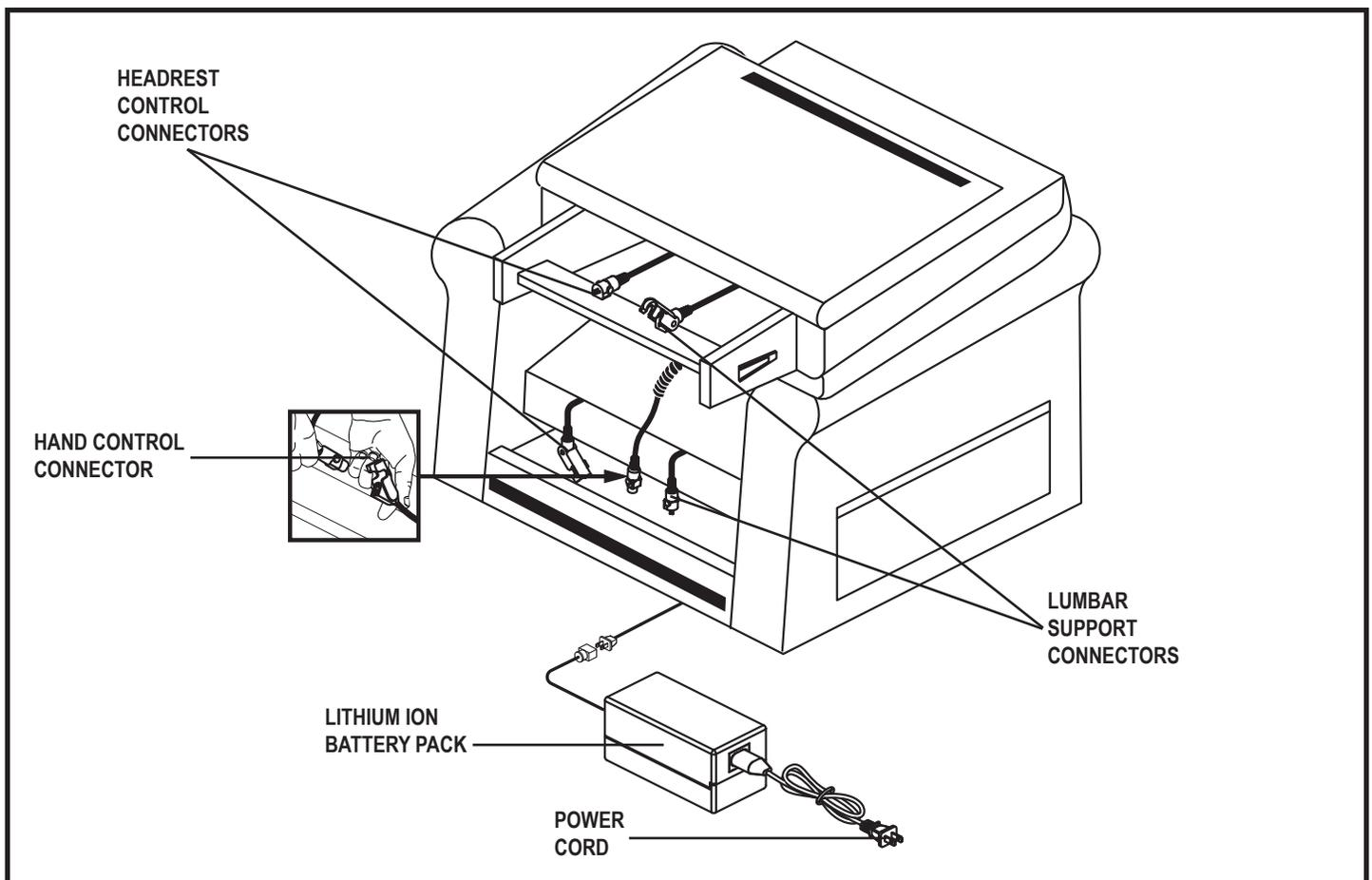
Figure 3. Chair Assembly - Power Transformer, Cords, and Connections
