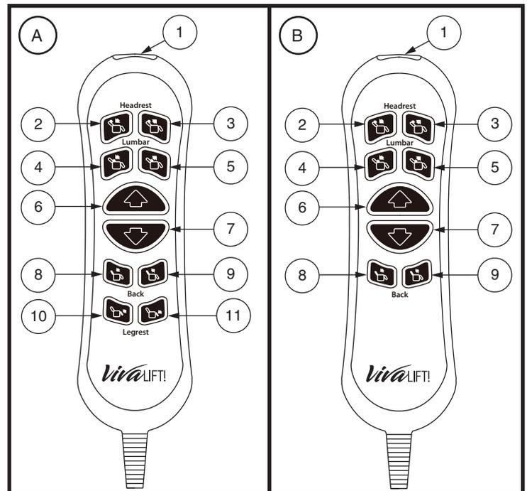
Figure 1. Hand Control - Styles A and B
